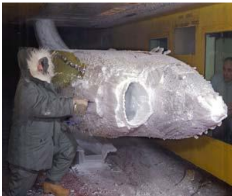
▲ Icing wind tunnel test
